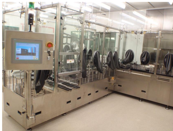
RABS filling line with freeze dryer
